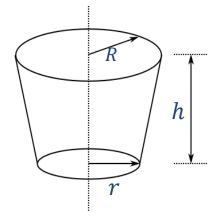
Maximize the volume of a bucket with a given surface of metal  $V = \frac{\pi h}{3} (R^2 + Rr + r^2)$  $S = \pi r^2 + \pi (R + r) \sqrt{(R - r)^2 + h^2}$
